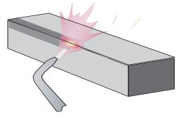
The surface to be hardened is heated continuously by means of a gas flame to approx.  $850^{\circ}C$  (pale-red colour), followed by cooling in air. The gas flame may be an ordinary oxyacetylene flame. The size of the blowpipe and the temperature of the gas are adapted so that the heating is accomplished in a few seconds.
