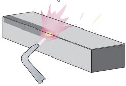
The surface to be hardened is heated continuously by means of a gas flame to approx. 850°C (pale-red colour), followed by cooling in air. The gas flame may be an ordinary oxyacetylene flame. The size of the blowpipe and the temperature of the gas are adapted so that the heating is accomplished in a few seconds. The flame hardened tool does not need to be tempered as this would cause a drop in hardness.
