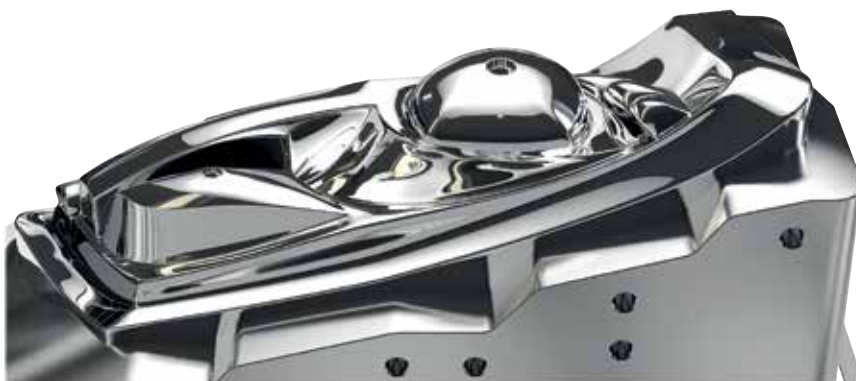
A highly polished mould for production of car headlights.
