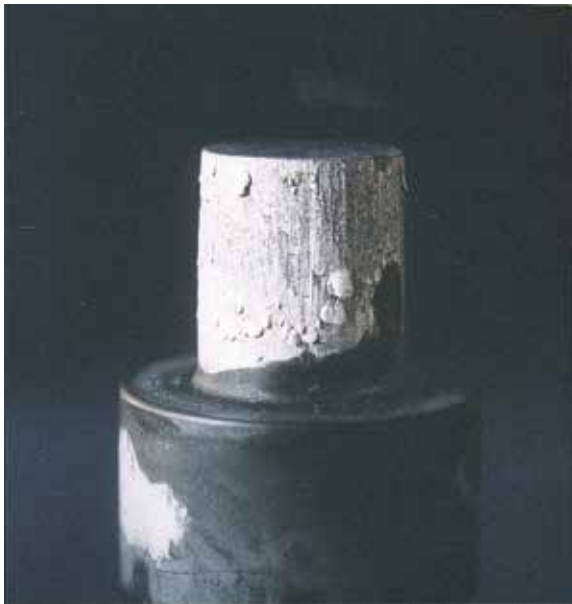
Soldering damage on a core pin
