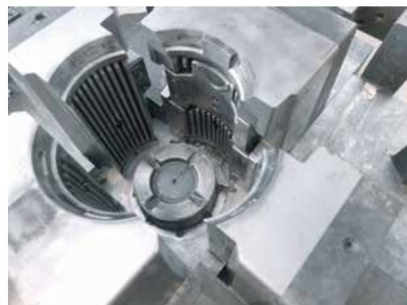
Cavity part for high pressure aluminium die casting.
