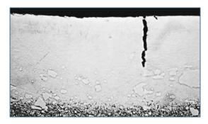
Photo 4. Surface of ASSAB XW-42 after rough spark EDM. The white layer is brittle and contains cracks.
