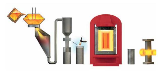
Figure 6. Schematic representation of the powder metallurgy (PM) route for producing tool steel.
