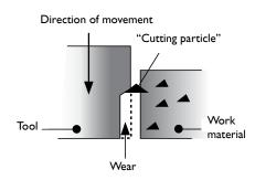
Figure 2 Schematic representation of abrasive wear.
