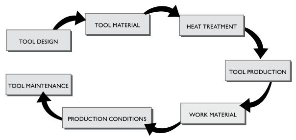
Figure 1. Factors influencing tool life in cold work application.
