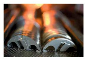
Sintering of powder compacted parts.
