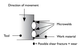
Figure 4. Schematic representation of adhesive wear.
