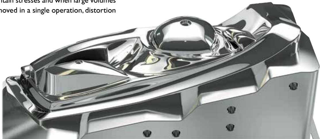
A highly polished mould for production of car headlights.
