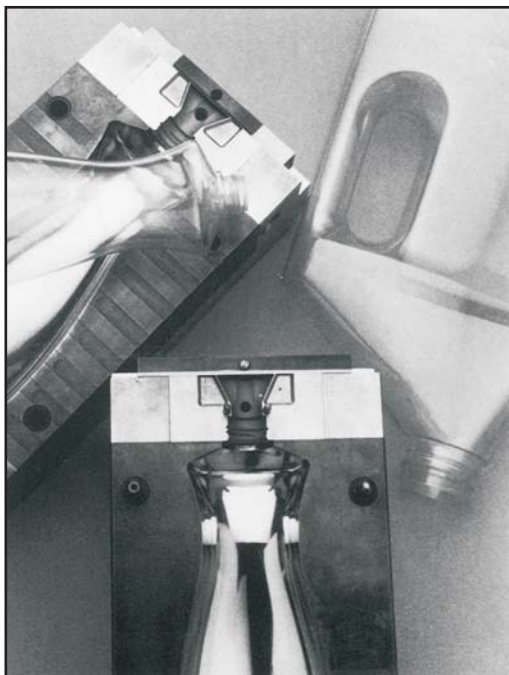
Two halves of a MOLDMAX beryllium copper blow mould.
